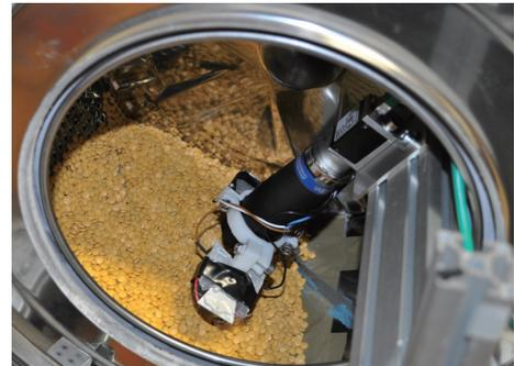
Figure 3: A rotating drum was used to simulate the movement of the tablets similar to the movement in real tablet coating machines.
