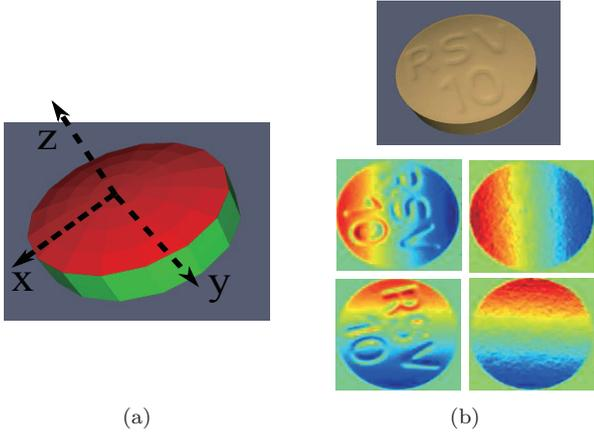
Figure 2: A simple 3D model used for the detection and out-of-plane rotation estimation of the tablets on the acquired images (a). A detailed 3D model of tablet’s surface including the information about the embossing (b). The detailed model is used for the estimation of the rotation of the tablet around its z-axis and for tablet side classification.
