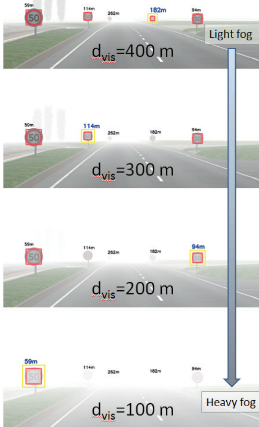
Figure 1. Traffic sign detection with increasing density of fog: BCT operating range decreases with fogginess.
