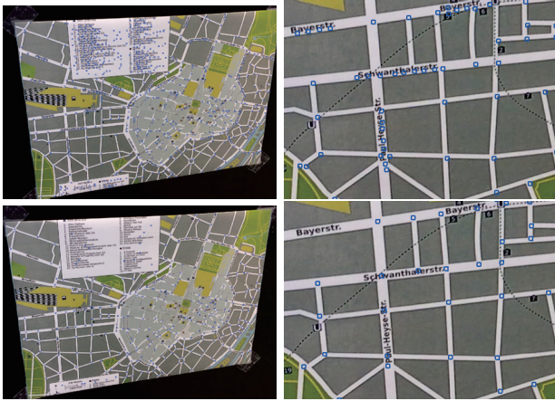
Figure 7. Intersection detection results (Blue points). Top: filter-based method of [12]. Bottom: Ours.
