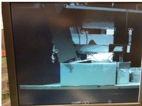
Figure 4: Harris Corner feature detected by our FPGA hardware method
