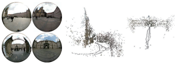
Figure 3: Randomized SfM tool [8]. 4,472 fish-eye images acquired by Nikon FC-E8 lens (left) were input into the pipeline resulting in several 3D models, the largest of them consisting of around 100 camera poses (right).
