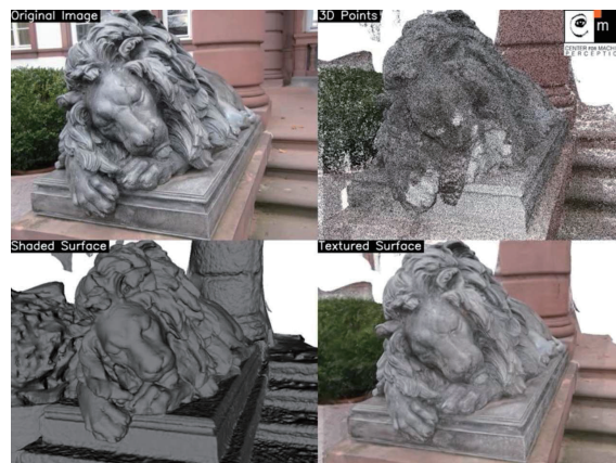
Figure 1: “One-button” reconstruction of LION dataset as seen from the viewpoint of one of the original images. Input image (top left), 3D points created during plane-sweeping (top right), resulting shaded mesh (bottom left), textured mesh (bottom right).
