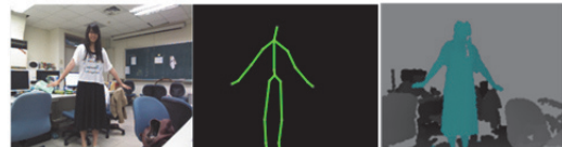
Figure 2. The color image, tracking human skeleton, and depth maps captured by Kinect
