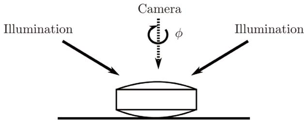
Figure 2. Illumination and camera setup. Camera view is parallel to the tablet rotation axis
