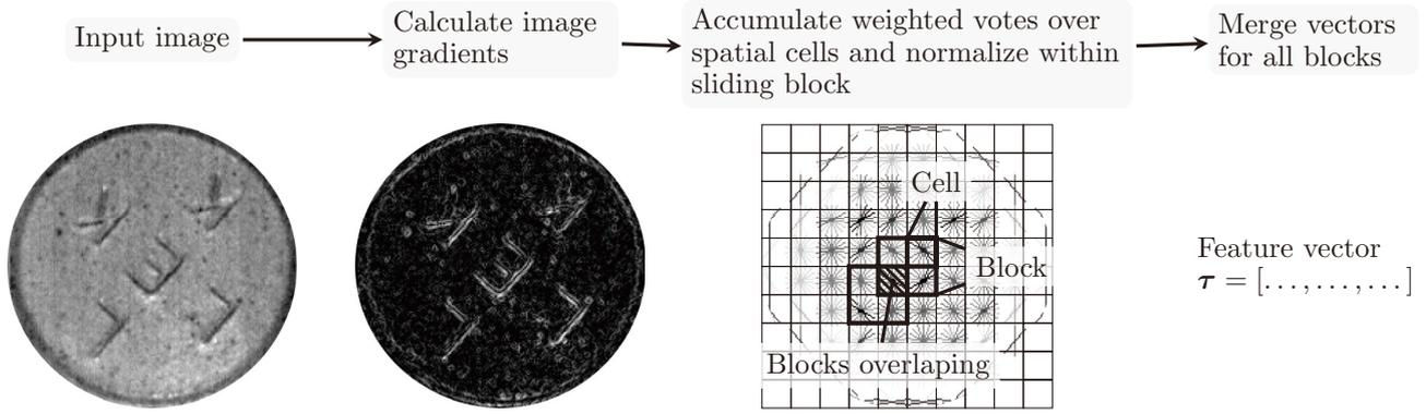
Figure 3. Histograms of Oriented gradients.
