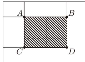
Figure 4. The value  $I(x, y)$  at any point  $(x, y)$  is the sum of all the pixels above and to the left of  $(x, y)$  inclusive,  $I(x, y) = \sum_0^x \sum_0^y i(x', y')$  - integral of pixel values within arbitrary rectangle  $ABCD$  is obtained by  $I(D) + I(A) - I(B) - I(C)$ .
