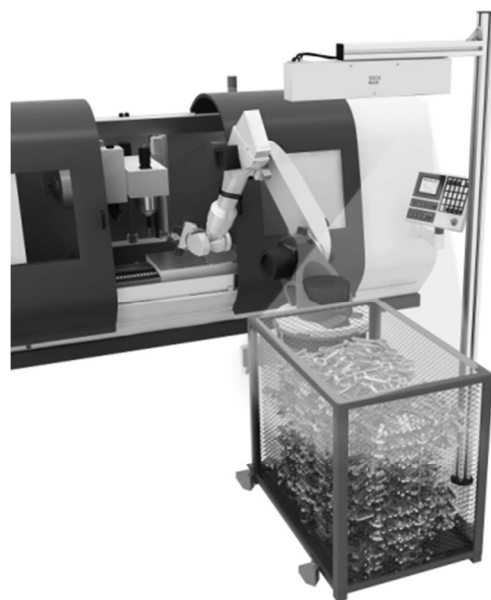
Figure 16. An illustration of a PLB bin picking system using the Scanning Ruler. 3D image data from the Scanning Ruler is used to control where the robot picks up an object.
