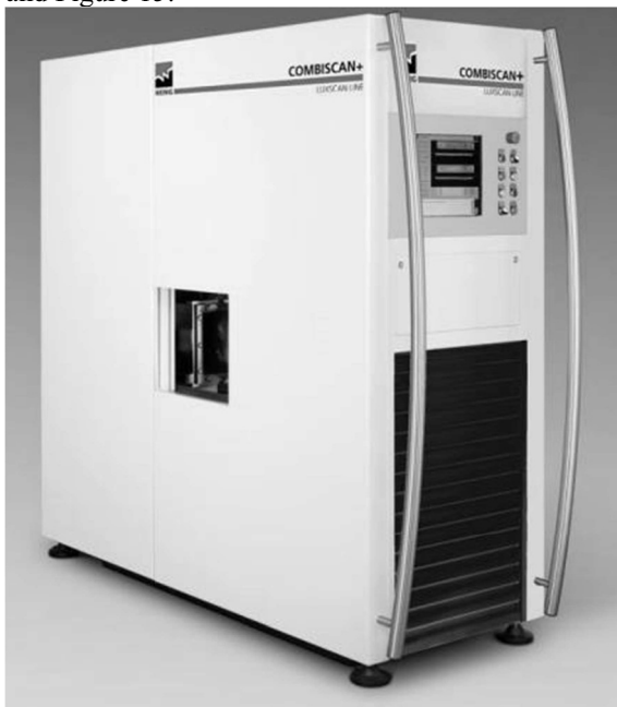
Figure 14. A board scanner from Weinig/Luxscan with 4 Ranger E cameras.
