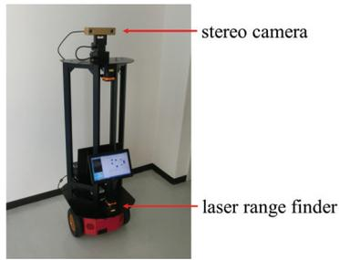
Figure 3. A mobile robot with a laser range finder and a stereo camera.
