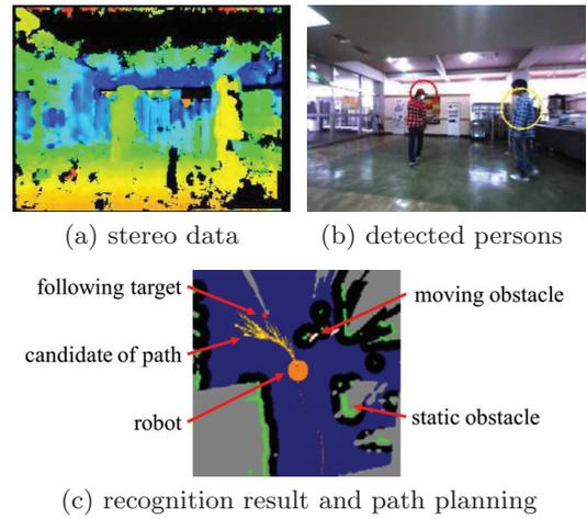
Figure 4. An example of scene recognition and motion planning.
