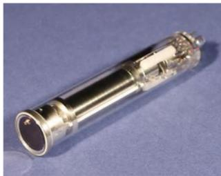
Figure 3. External view of the 2/3-inch HARP tube.
