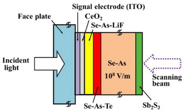
Figure 2. Target structure.
