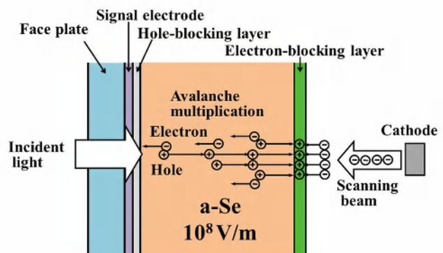
Figure 1. Operational representation of the HARP tube.
