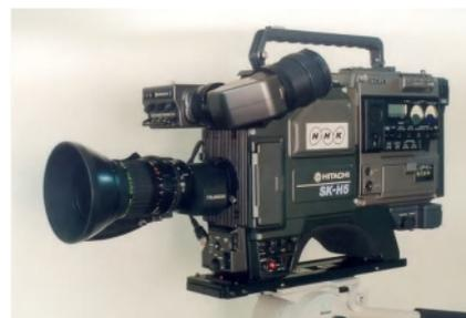
Figure 5. Appearance of the three-tube HARP camera.
