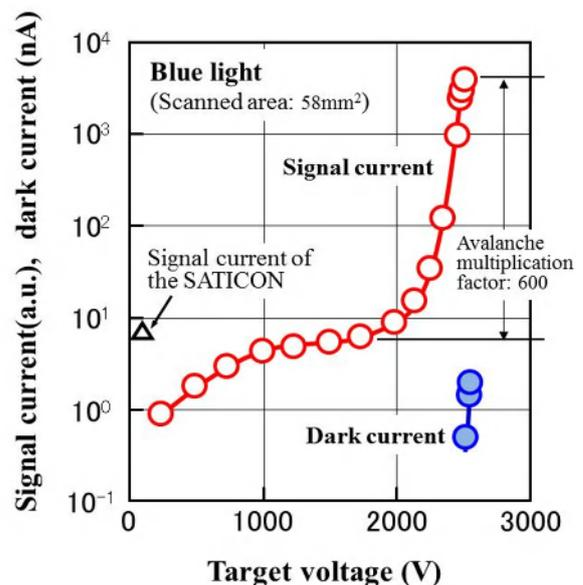
Figure 4. Signal current and dark current versus target voltage.
