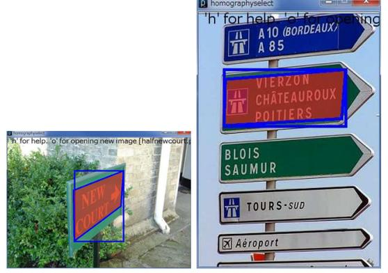
Figure 2. The rectangular quads indicate the traditional area selected by a click-and-drag interaction. The perspective quad indicates the perspective sub-rectangle selection.
