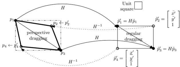
Figure 3. Perspective dragging: The user selects  $p_1$  and drag  $p_3$ . The system maps  $p_1$  and  $p_3$  to  $p'_1$  and  $p'_3$  using the predefined convex quad-to-square homography  $H$ . It then makes a rectangular bounding box  $(p'_1, p'_2, p'_3, p'_4)$  with opposite corners  $p'_1$  and  $p'_3$ , and maps back  $p'_2$  and  $p'_4$  to the image coordinate system using the inverse square-to-convex quad homography  $H^{-1}$ .
