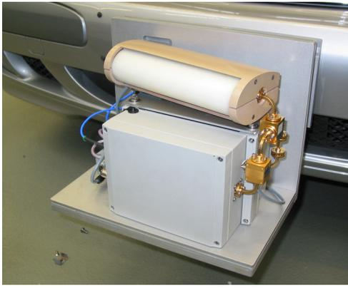
Figure 7. Experimental imaging radar sensor.
