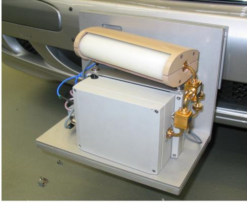
Figure 7. Experimental imaging radar sensor.
