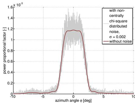
Figure 3. Result of the convolution and the addition of noncentrally chi-square distributed noise.
