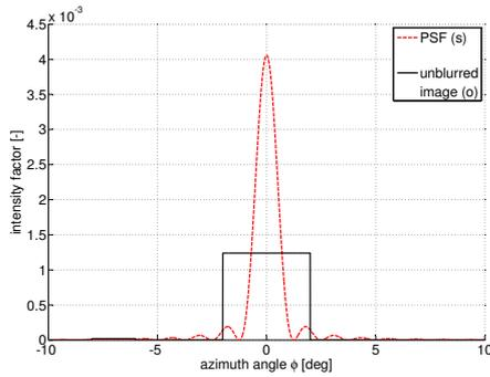
Figure 2. Unblurred image and point spread function (PSF) used for simulation.
