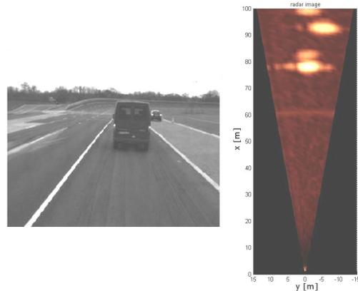
Figure 1. Car in the image of an automotive scanning radar sensor.
