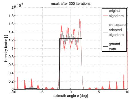
Figure 4. Result from the adapted Lucy-Richardson algorithm compared to the result from its original form. Note the still detectable small target at  $-7^\circ$ .
