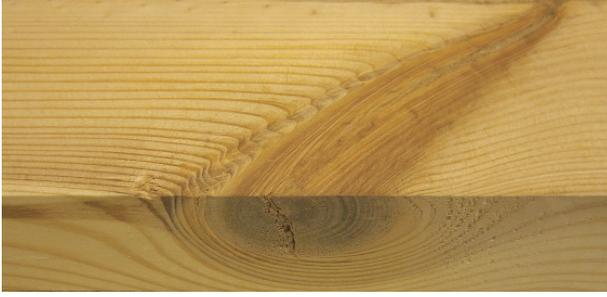
Figure 1. Grain behavior around a knot.
