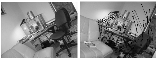
Figure 2. Pair of images and identified key points with displacements described by affine transformation.
