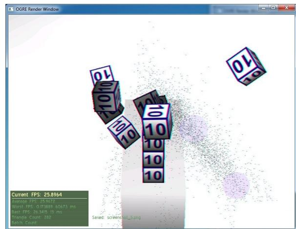
Figure 1. A screenshot of the interaction. A wall of dice is toppling over after colliding with a person's hand, represented by two pink spheres; dots are filtered points from the range camera before outlier removal.
