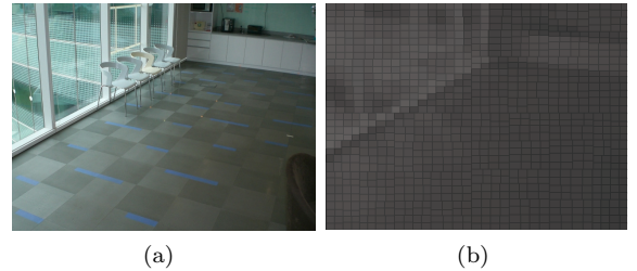
Figure 2. Quadtree Decomposition of the image. At each step, the four regions have the same entropy value, the image is coded using 1024 patches. (a) Original Image (b) Codified image.
