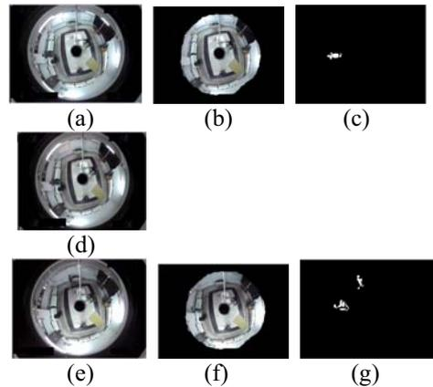
Figure 8. The experimental results in the case of turning partial light on and off. (a) Input image before light is off. (b) Background before light is off. (c) Foreground before light is off. (d) Input image at the instant of turning light off. (e) Input image after light is off. (f) Background after light is off. (g) Foreground after light is off.
