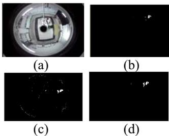
Figure 6. Binarization results using different thresholds: (a) Original image. (b) Noise threshold (fixed at 35). (c) Noise threshold (fixed at 20). (d) Noise threshold (fixed at 20) +  $I_{diff}$  (dynamic).
