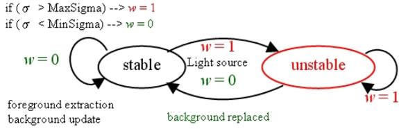
Figure 1. The state transition diagram for on and off light detection.
