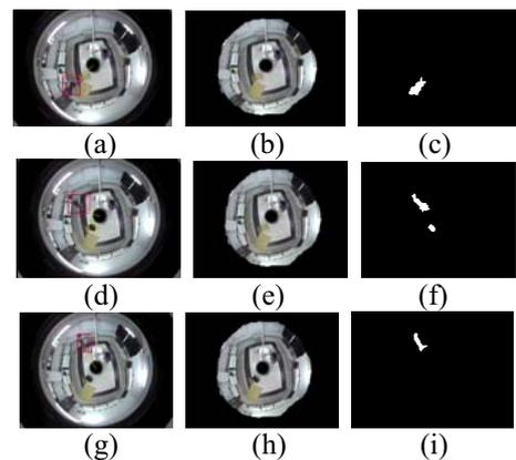
Figure 9. The experimental results of abandoned object detection and removal. (a) Input image before object is abandoned. (b) Background before object is abandoned. (c) Foreground before object is abandoned. (d) Input image after object is abandoned. (e) Background after object is abandoned. (f) Foreground after object is abandoned. (g) Input image after abandoned object is removed. (h) Background after abandoned object is removed. (i) Foreground after abandoned object is removed.
