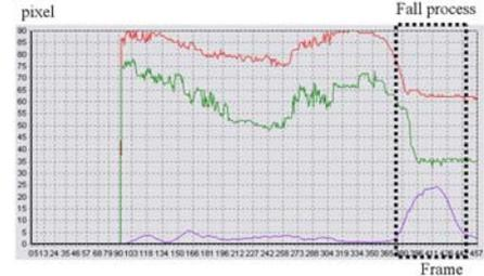
Figure 4. A typical result of tMHI-based feature when radially inward fall occurs.
