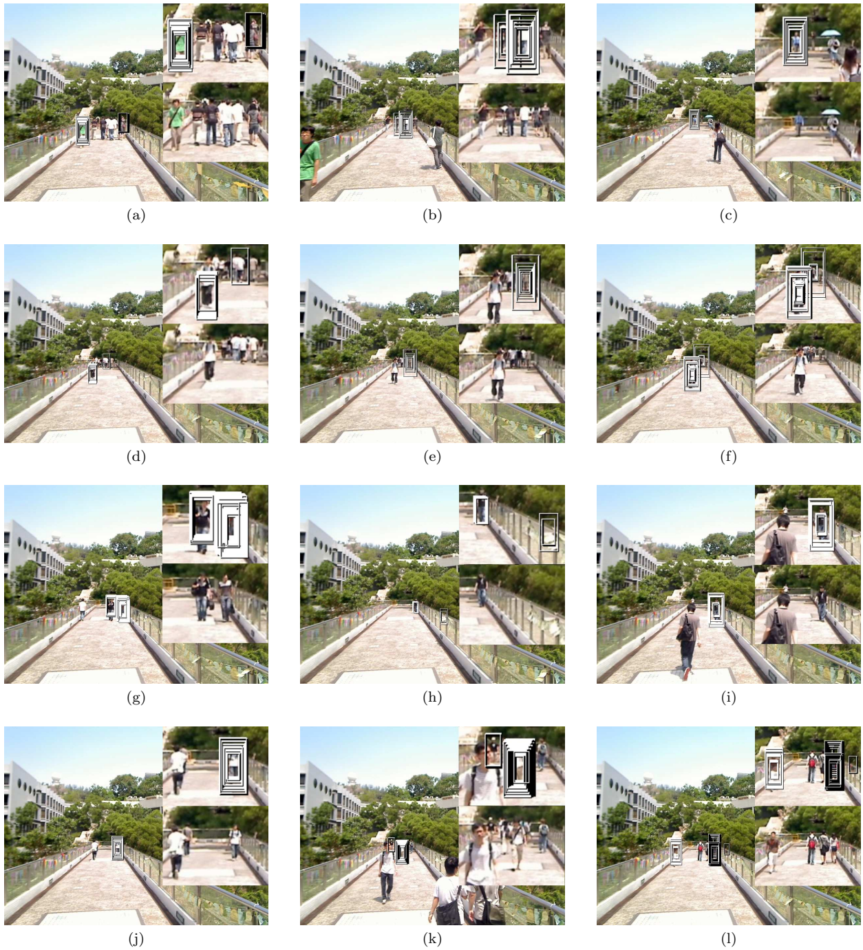
Figure 3: (a)-(l): Detection result of our proposed algorithm on a video sequence taken at a long bridge. Detection windows that are classified as pedestrians are represented using white rectangles. The embedded image on the top right hand corner on each figure is a close-up of the detection results. The images at lower right hand corner are close-ups of original video frames.
