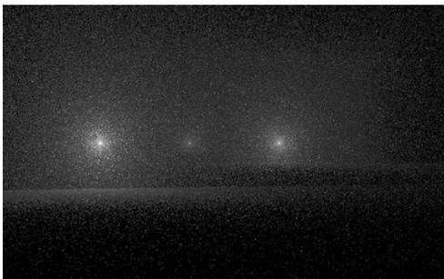
Figure 1: Simulation of three point sources in fog (35m, 200m and 80m from left to right)
