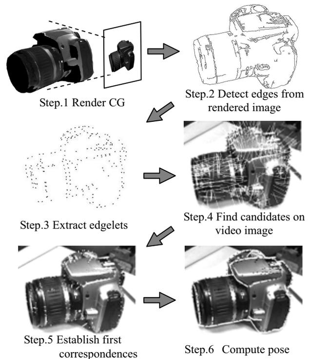
Figure 1: Pose estimation using textured 3D model.
