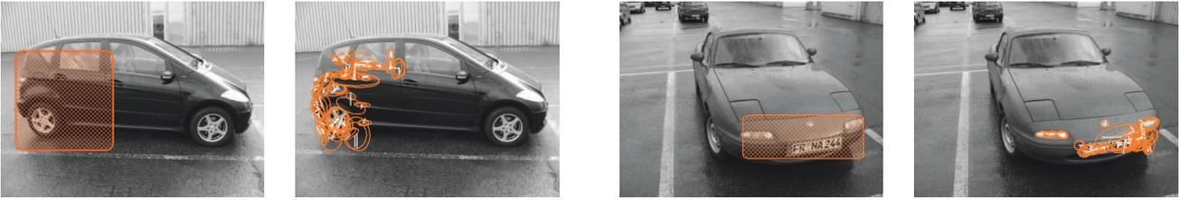
Figure 3: Object parts in their most frontal view. We use histograms based on interest points in order to robustly describe the visual appearance of object parts.
