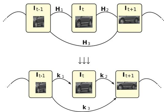
Figure 4: Using the foreshortening factor leads to a directed graph with which we can determine the part which is shown in its most frontal view.
