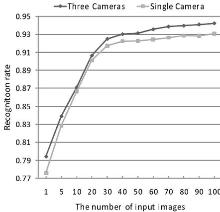
Figure 7: Changes of recognition rate in terms of the number of input patterns.
