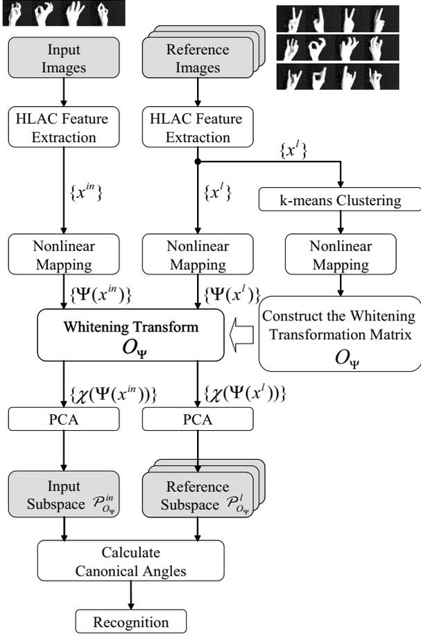
Figure 3: The flow of the proposed method.
