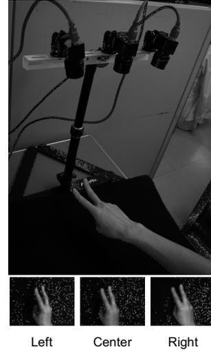
Figure 4: Multiple cameras system and the multiple view images captured from the three cameras.
