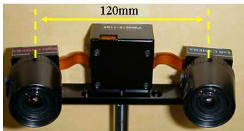
Fig.6 Photograph of stereo sensing module
