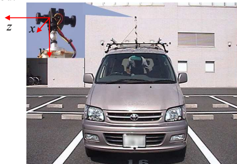
Figure 1. A full-view image sensor and a hybrid GPS sensor are installed on a vehicle to acquire data for route map building.
