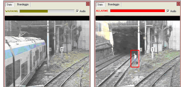
Fig. 5: left: allowed movement; right: alarm.
