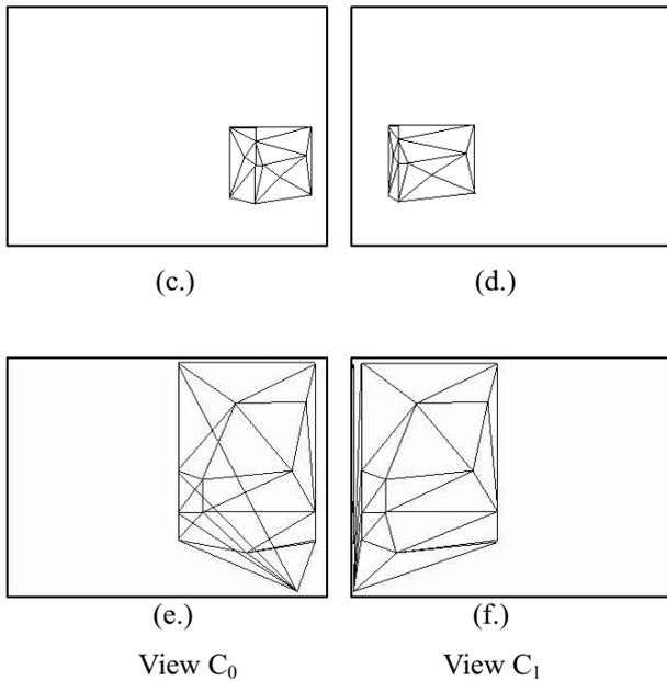
Figure 5. The triangle dividing. Top: the triangle patches of the object from viewpoints. Bottom: the triangle patches of the background from viewpoints.
